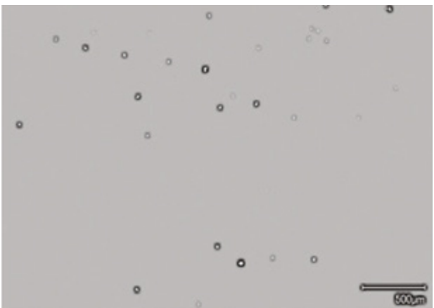
Figure 5, 6: Micrographs show the impact of addition of CEVO®-process B-3680 on dispersion of 2% carbon black agglomerates in HDPE. The left image contains no additive; the right image an addition of 0.5%.
